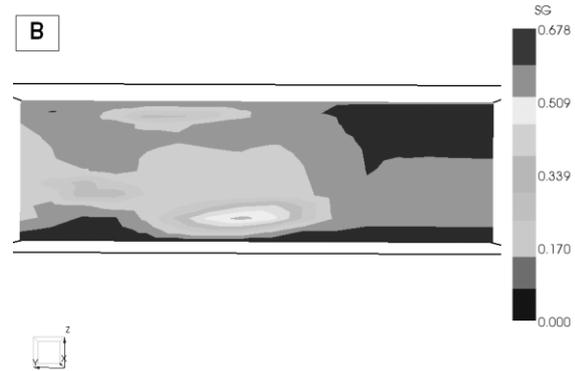
**Fig 4 b) North-South section of gas saturation in "Nikwa-Modrzejów" overburden strata [18]**
