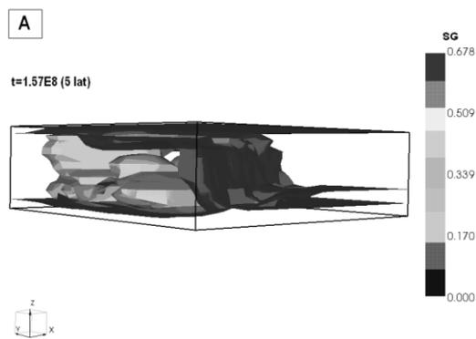
**Fig. 4 a) 3D projection of gas saturation in "Nikwa-Modrzejów" overburden strata [18]**
