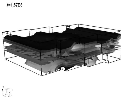
**Fig. 5 a) 3D projection of gas saturation in "1 Maja" overburden strata [18]**
