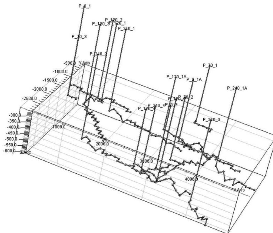
**Fig. 1 Model of ventilation system built in Eclipse [11]**
