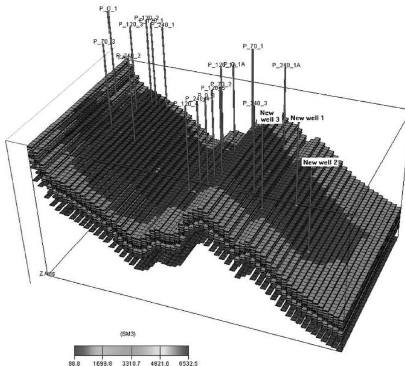
**Fig. 2. methane saturation in model cells [11]**
