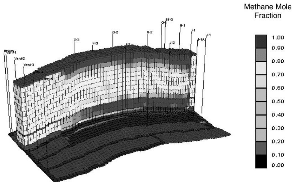
Fig.3. A vertical cross section of the subsided strata reservoir and the Pittsburgh coalbed layer 630 days after the start of mining [15]
