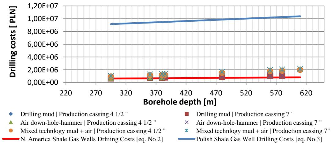
**Fig. 5. Drilling costs of shallow wells (<1000 m. dots) in comparison with deep shale gas wells cost (lines)**
