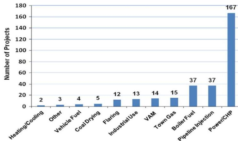
Fig 2. Global CMM projects according to M2M [5] after Karacan et al. [6]
